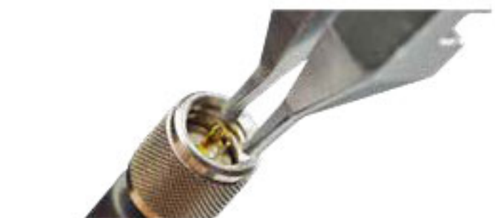
7292MI micro-mini end cutter is used to cut a ground wire inside a mini connector.
