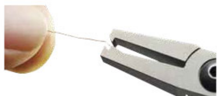
202A cut and clench tools leave a swaged, bent lead that clenches the PCB.
