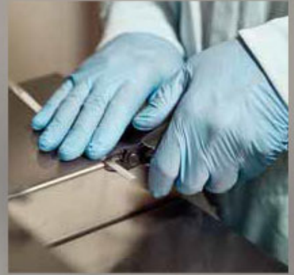
8150M2 cutter used to trim multiple stents thanks to the modified hardened cutting heads.
