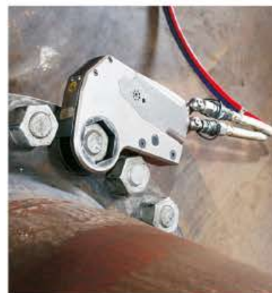
alkitronic® H-AX , when fitting a flange in plant construction.
